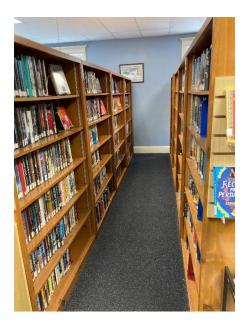
The facility has poor collection accessibility due to shelving height and insufficient aisle spacing. Shelving should be at least 42 inches apart for ease of use by wheelchair bound citizens.
